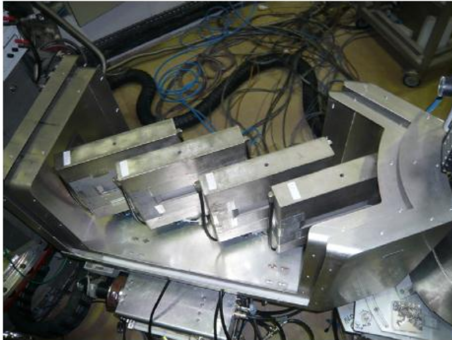
Fig. 2. View of the first "arm" of ZETA in the absence of the double \mu -metal shielding. The two pairs of RF flipper coils are tilted w.r.t. the beam axis by an angle of 70^\circ , showing the high flexibility of the setup.
